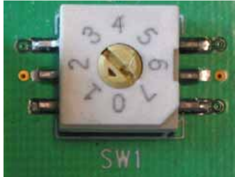
Figure 3-21. Address Switch SW1 on the Expansion Shelf
